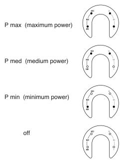
If "P max" maximum appliance operating power has been selected, adjust the thermostat dial (Fig. 2) to the desired comfort temperature, from  $42^{\circ}F(x)$  and  $95^{\circ}F(5^{\circ}C)$  and  $35^{\circ}C$ ).
